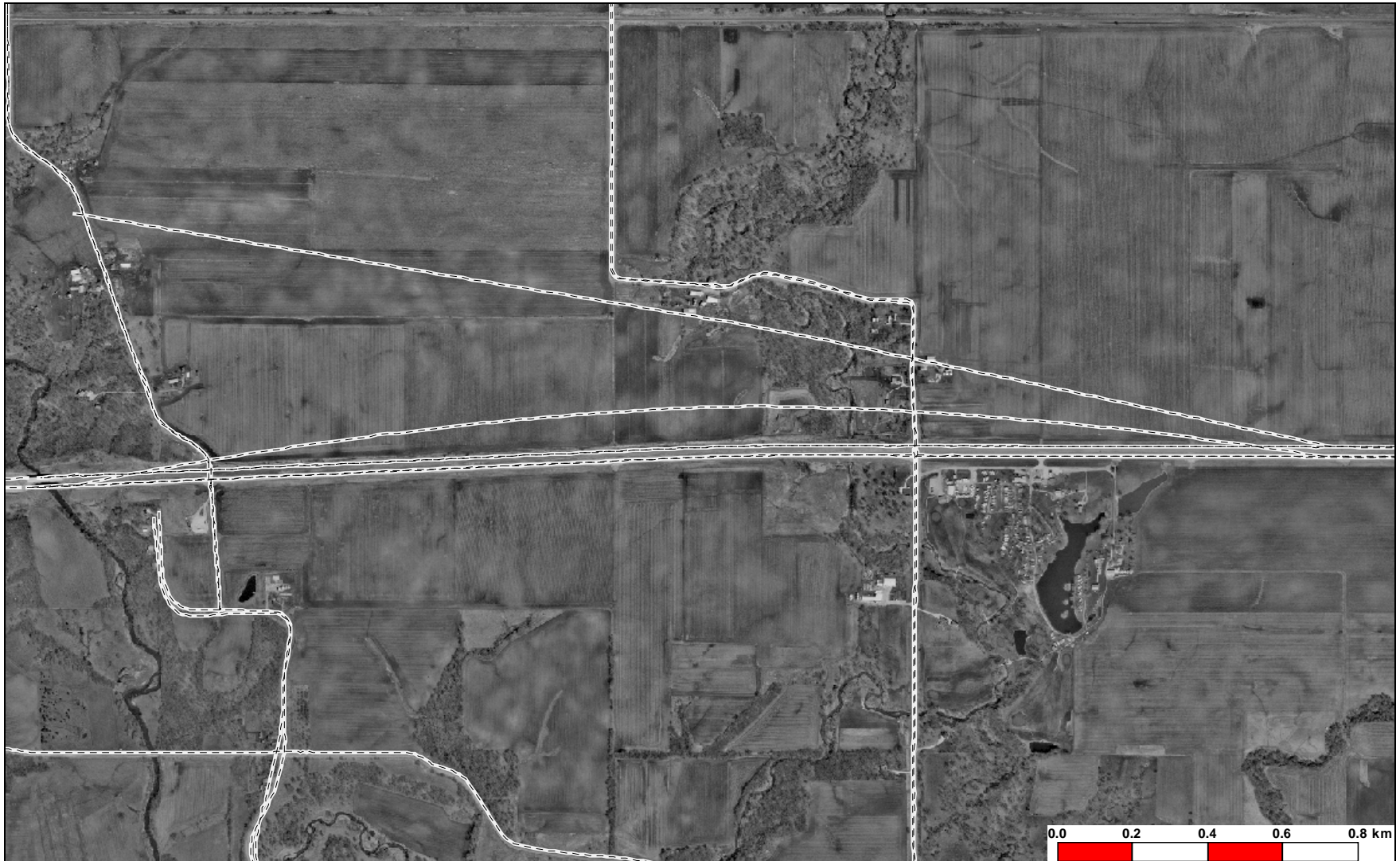
Figure 5-6 Videolog DGPS Measurements between Nevada and Colo along US 30
