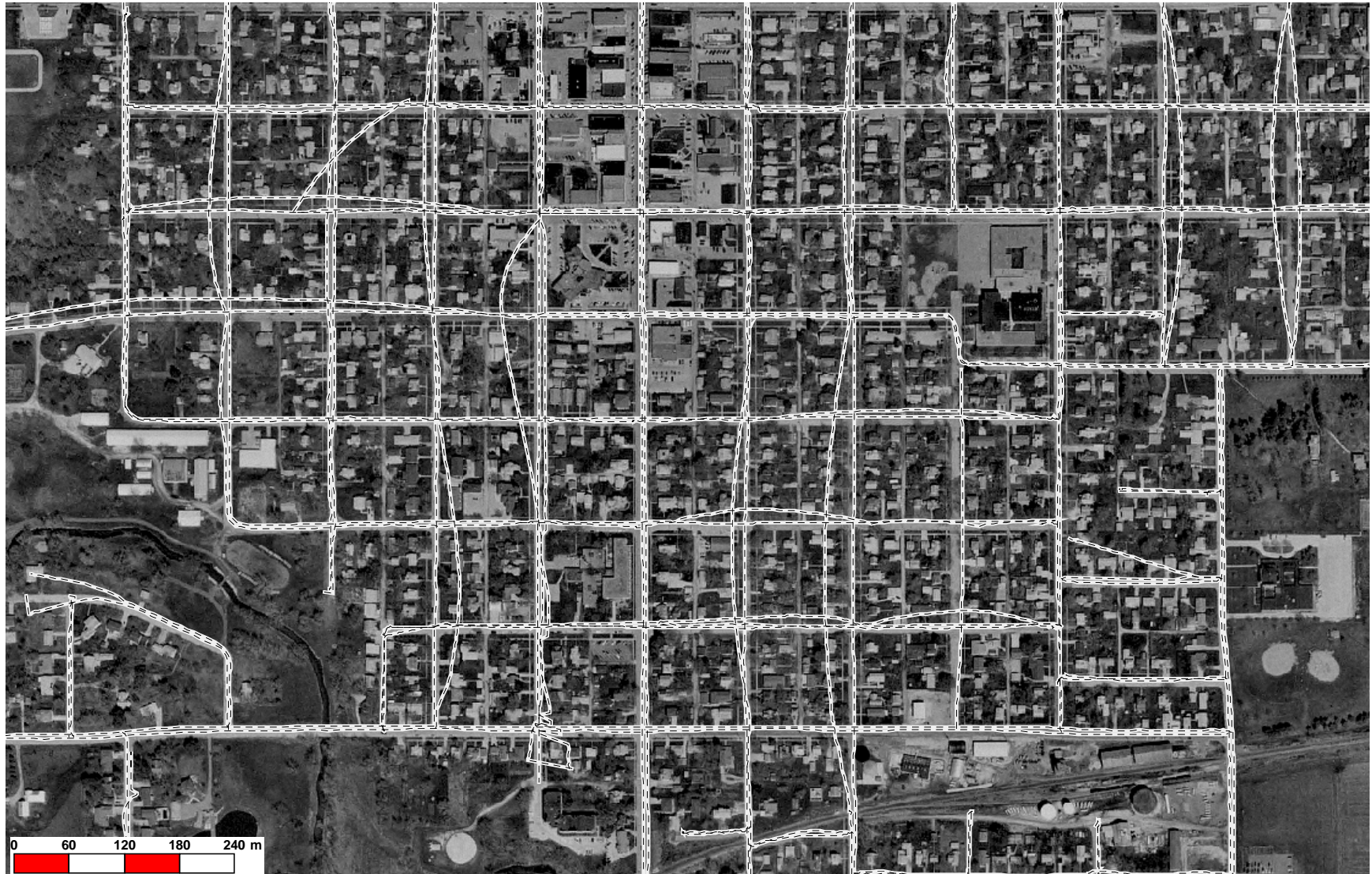
Figure 5-5 Videolog DGPS Measurements in Nevada
