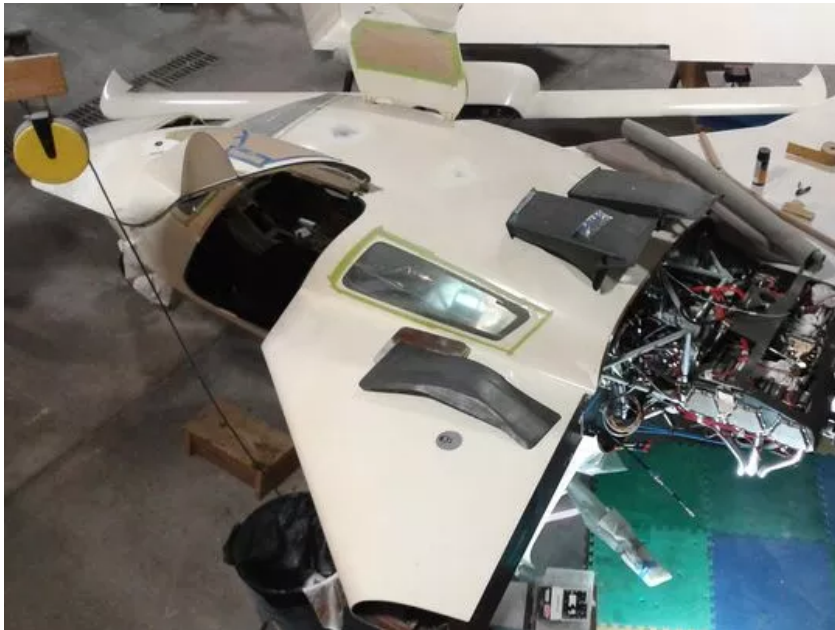
John Tvedte’s Velocity XL under construction will have a 31-foot wingspan, carry up to five people and cruise at 200 MPH. It features a “pusher” configuration in which the engine and prop are behind the cabin, which John says is a cleaner aerodynamic design. (Photo: Dick Hakes / Special to the Press-Citizen)
