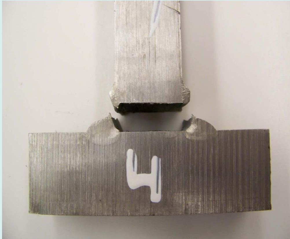
Photo 32 SAW Single Pass Fillet Fracture
