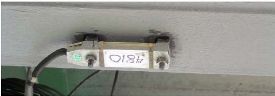
(b) Photograph of a strain gage installation on CFRP plate
