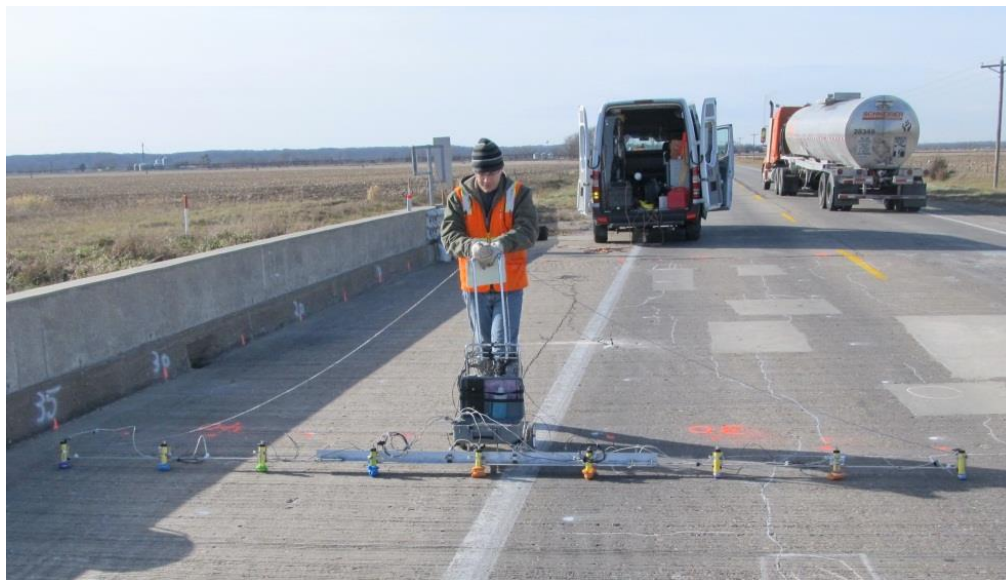
Figure 2.4. Measuring half-cell potentials with the nine-cell rolling test frame.
