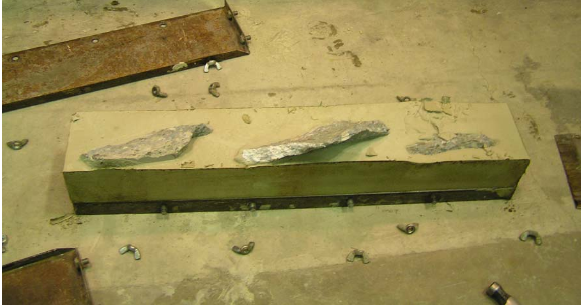
Figure 3.7. Mockup duct embedded in grout beam.
