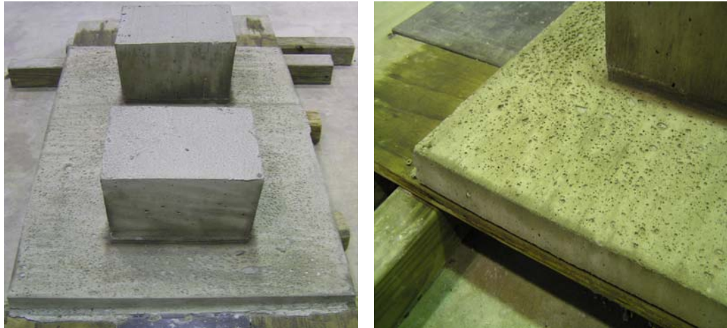
Figure 3.4. Stud pocket and haunch mock-up after form removal.
