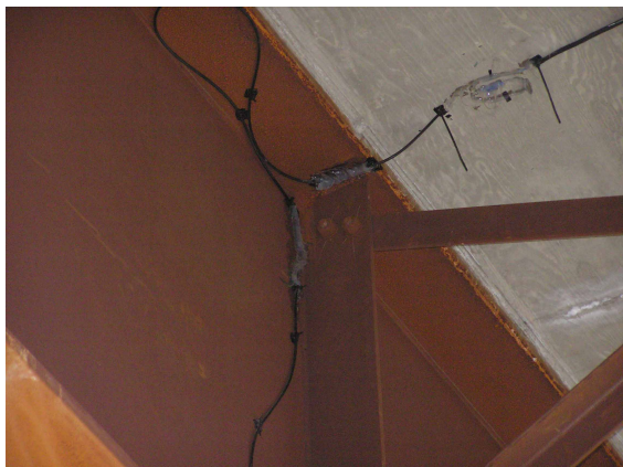
d. Two FBG Sensors for Monitoring Localized Weld Strains
