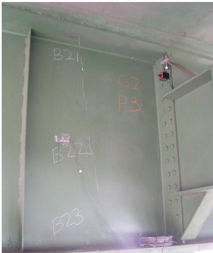
Figure 22. Strain gages B21, B22 and B23 on Girder 2 to assess flexural behavior near Pier 3.
