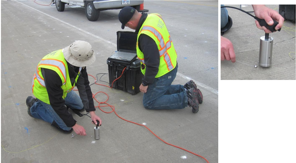
Figure 5.4. Collection of Impact-Echo data at distinct testing points using single-transducer IE unit.
