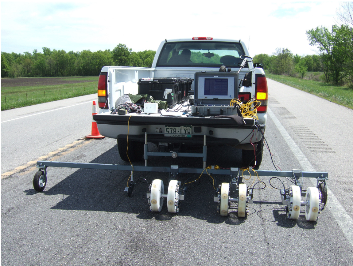
Figure 5 – Vehicle Mounted BDS-IE-SASW Transducer Alignment for an IE test on one wheel and an SASW test between the wheel pair spaced at 6 inches apart for asphalt delamination (debonding) detection by velocity decreases. Note that for Bridge Deck Scanning the spacing can be increased to 1 ft or 2 ft between each pair of wheels to provide for ½ lane to a full lane scan per pass with tests ~ every 6 inches.
