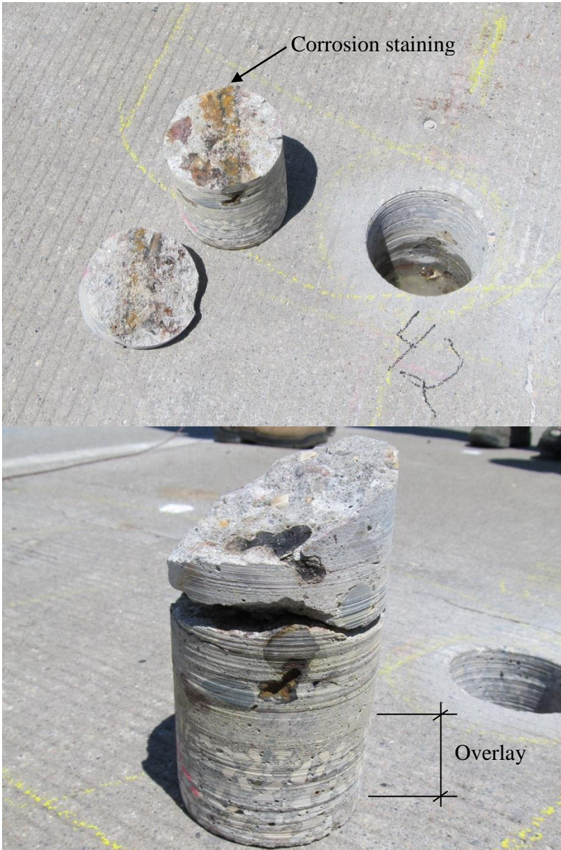
Figure 2.11. Core sample with evidence of horizontal cracking/delamination along the plane of reinforcement due to corrosion of the reinforcing. Note smaller coarse aggregate in overlay visible in bottom photograph.
