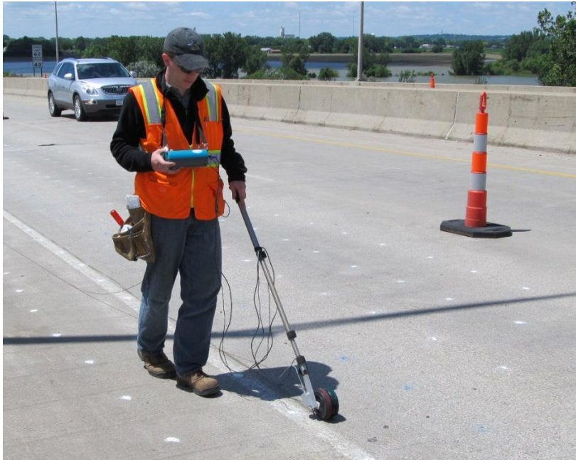
Figure 6.5. Measuring half-cell potential using a CSE integrated with a rolling wheel.
