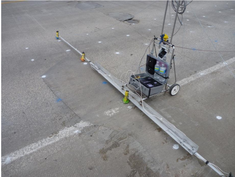
Figure 6.4. Rolling cart with five CSEs and datalogger, used for half-cell potential measurements.
