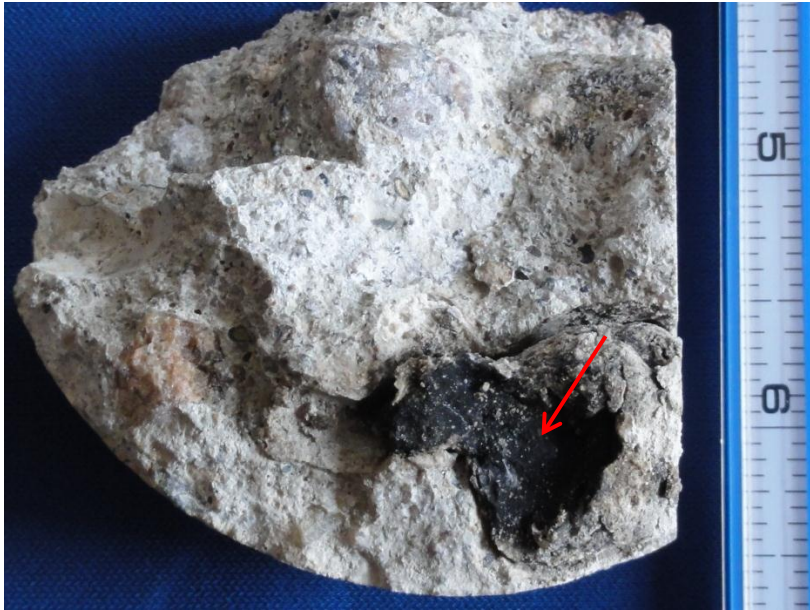
Figure 10. Core 42; large lump of industrial waste containing reactive glass embedded at the bottom of the base concrete.
