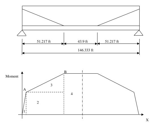
Moment-Area Method -- Point A is the transfer point, Point B is the harp point  $M_A = (2211.9 \text{ kip})*(27.357 \text{ in} - 13.898 \text{ in}) = 29,768.77 \text{ kip*in}$
