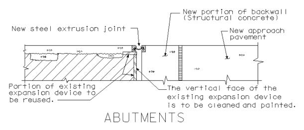
Figure 12.1.9.1.7. Backwall replacement with remodeled expansion joint
