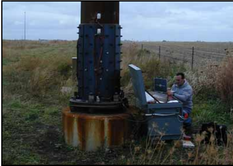
Figure 2.7 – View of data acquisition box at the Retrofit tower along US-18 in Clear Lake, IA
