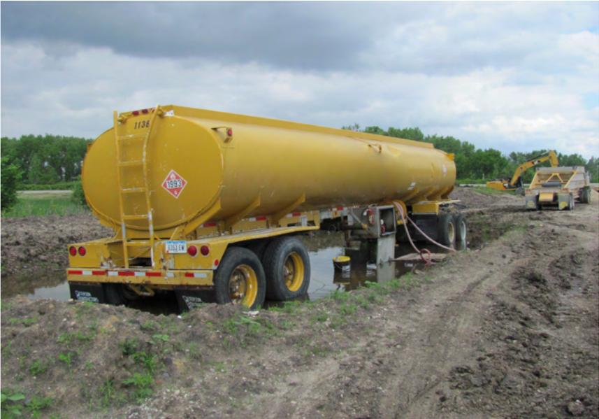
**This fuel tank has an earth berm built around it to act as secondary containment.**
