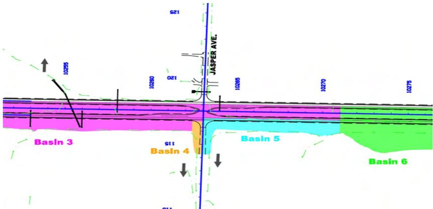
Plan sheet showing color coded drainage basins and discharge points
