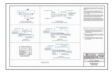
There are many different runout typical details available to fit many different situations (single vs. multiple lifts, notched vs. full runouts, etc.).
