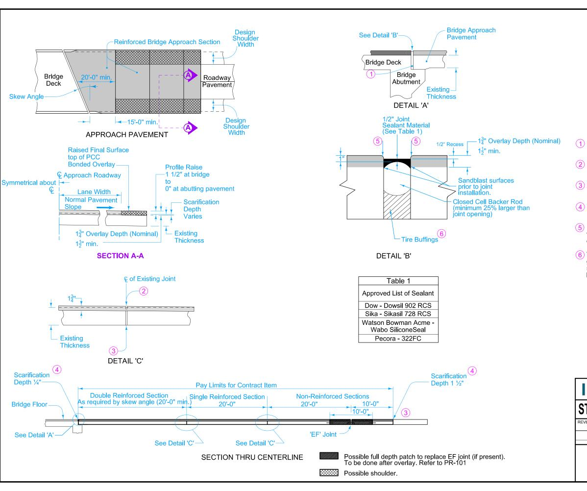
Remove all HMA within pay limits if present. Removal of previous HMA overlays will be incidental to "Deck Overlay" and will not be paid for seperately. Full depth patch maybe required to remove HMA, see project plans.
