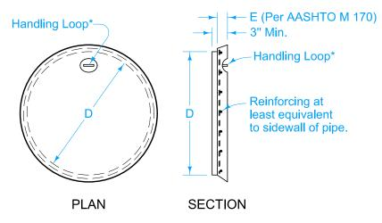
\*The handling loop may be omitted when the cap is placed in a buried installation.
