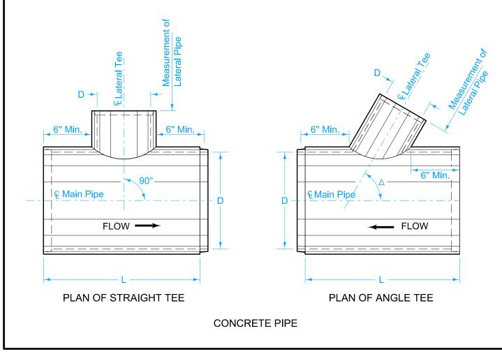
Tees may be required in any size from 12 inch diameter to 48 inch diameter (in 6 inch increments) on main pipe culverts equal to or greater in diameter than that of the tee. Angle tees may be required in any delta angle (of 5 degree increment) between 45 and 90 degrees. Consider a tee section delta angle 90 degrees (straight tees) unless noted otherwise in the project plans
