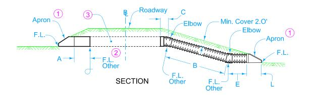
A = Concrete Pipe Length B+C+E = Corr. Pipe Length
