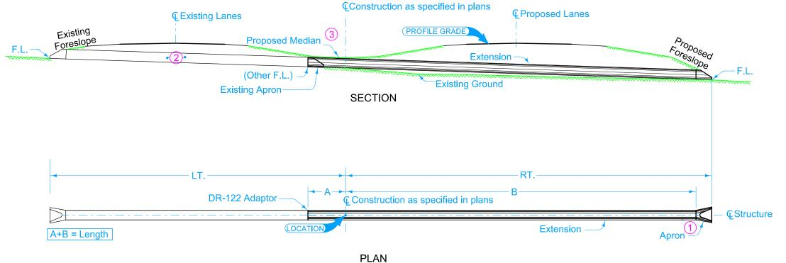
Extend on line of existing structure to Lt., Rt. or both as specified. Adapters may be required, see DR-122.
