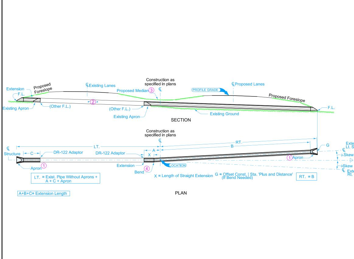
Extend in the direction specified with skew measured from centerline of existing structure. Dimension Rt. or Lt. is measured at C of pipe along laying length.
