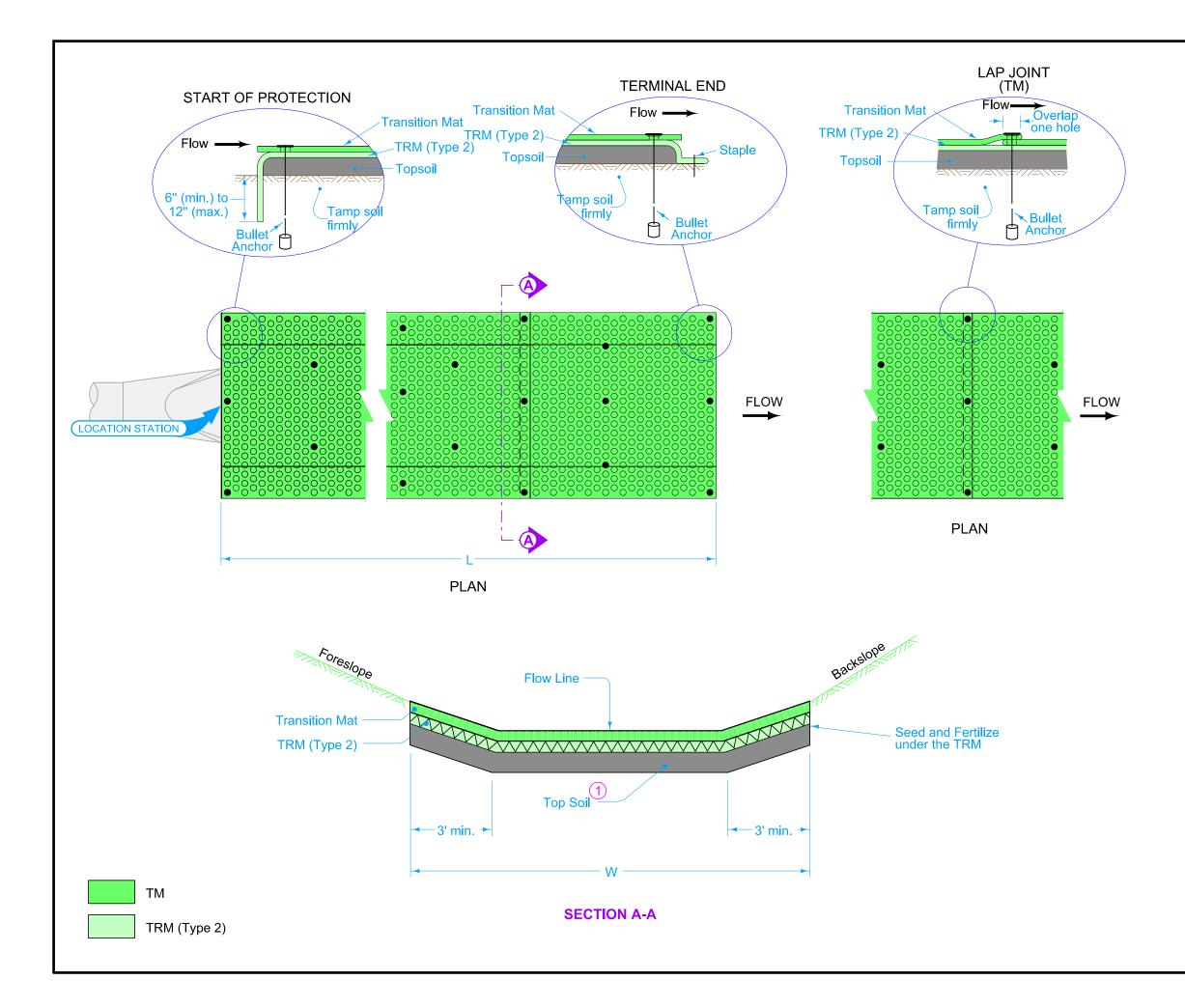
Refer to Standard Road Plan EC-104 for the placement of the TRM.
