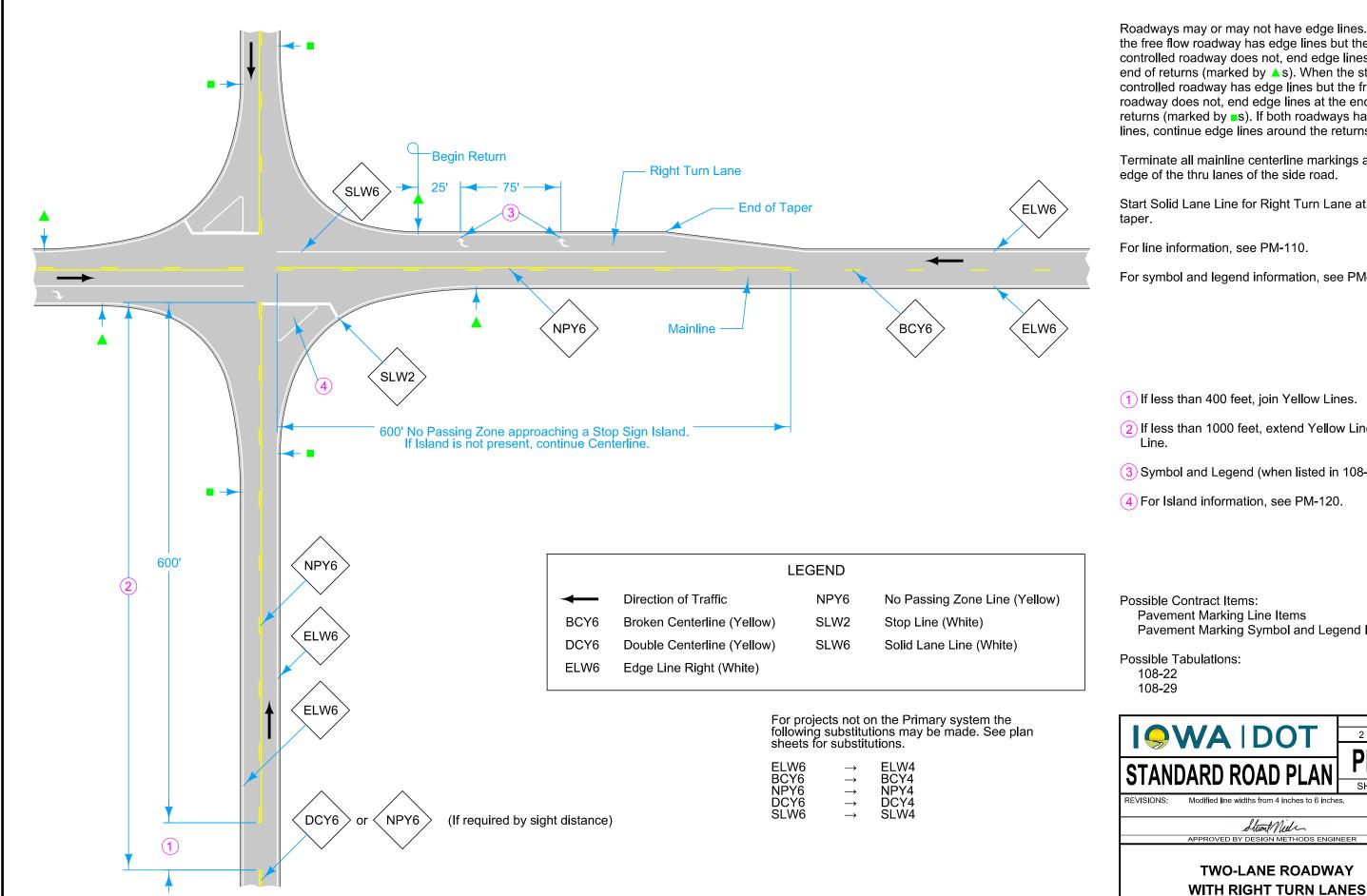
Roadways may or may not have edge lines. When the free flow roadway has edge lines but the stop controlled roadway does not, end edge lines at the end of returns (marked by \( \Lambda \) s). When the stop controlled roadway has edge lines but the free flow roadway does not, end edge lines at the end of returns (marked by s). If both roadways have edge lines, continue edge lines around the returns.
