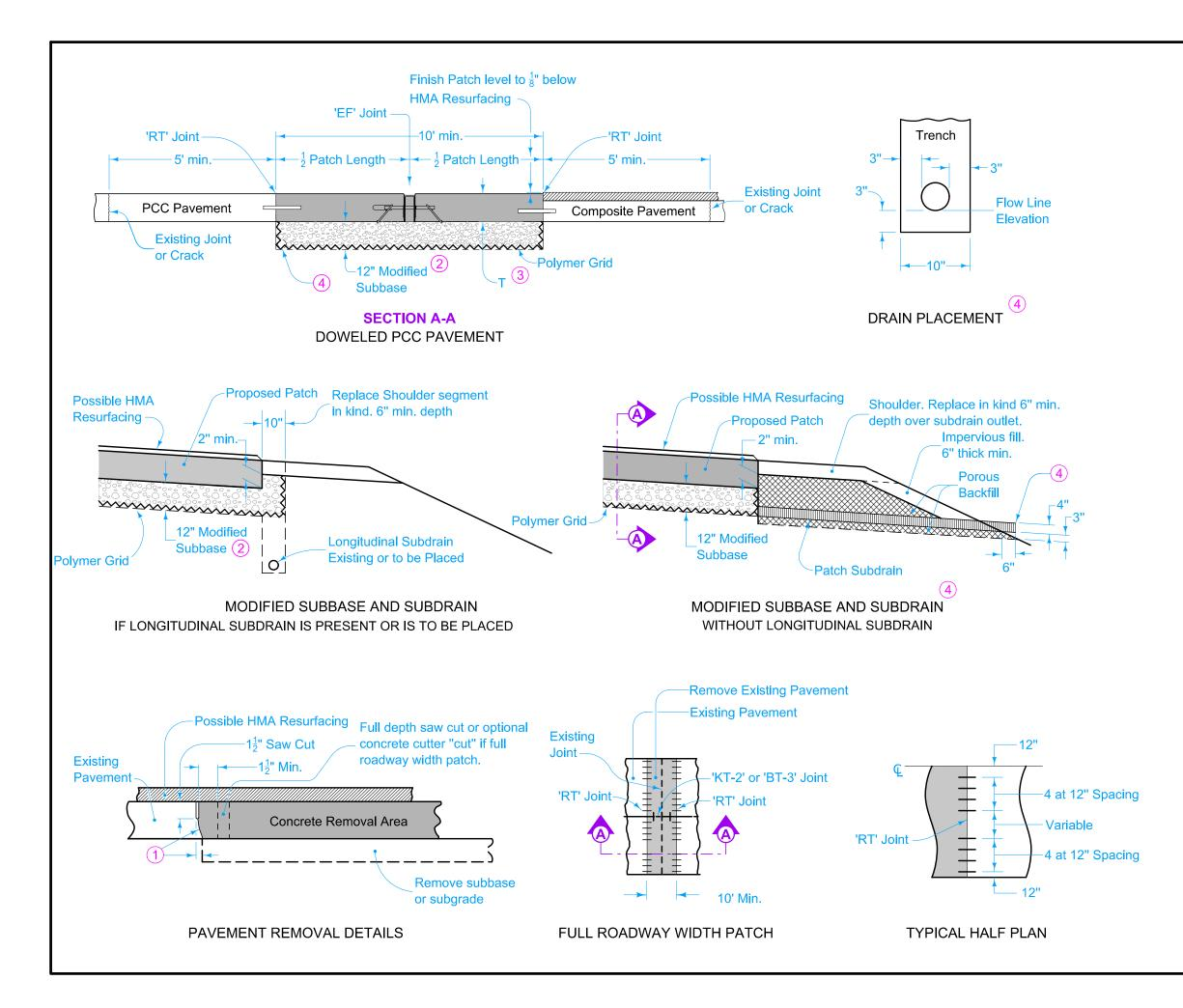
Place Full Depth Patch with 'EF' Joint after the final lift of asphalt has been placed. Porous Backfill and Subdrain may be placed prior to construction of resurfacing of shoulders.
