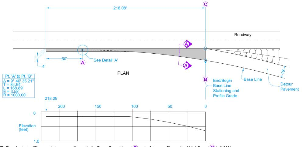
NOTE: The algebraic difference between profile grade for Ramp Base Line at B and relative profile grade of Mainline at C is 0.63%.
