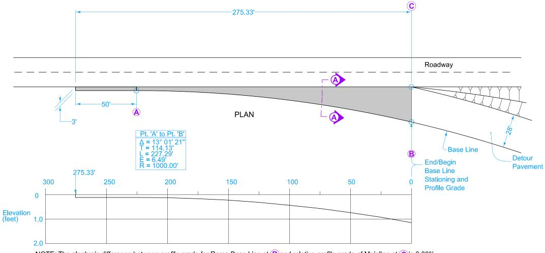
NOTE: The algebraic difference between profile grade for Ramp Base Line at B and relative profile grade of Mainline at c is 0.88%.
