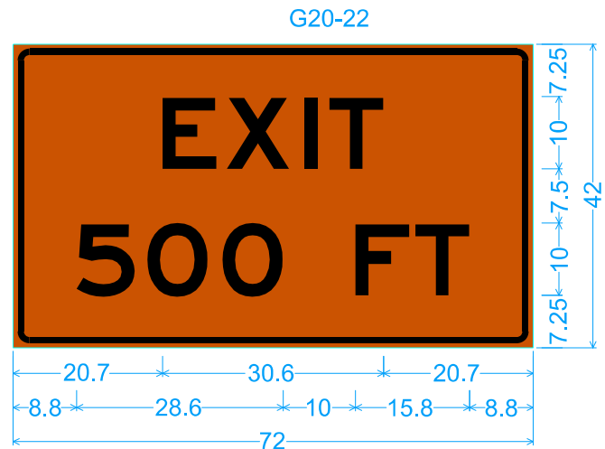
G20-22 2.25" Radius, 0.88" Border, 0.63" Indent, Black on Orange; [EXIT] E 2K; [500 FT] E 2K;
