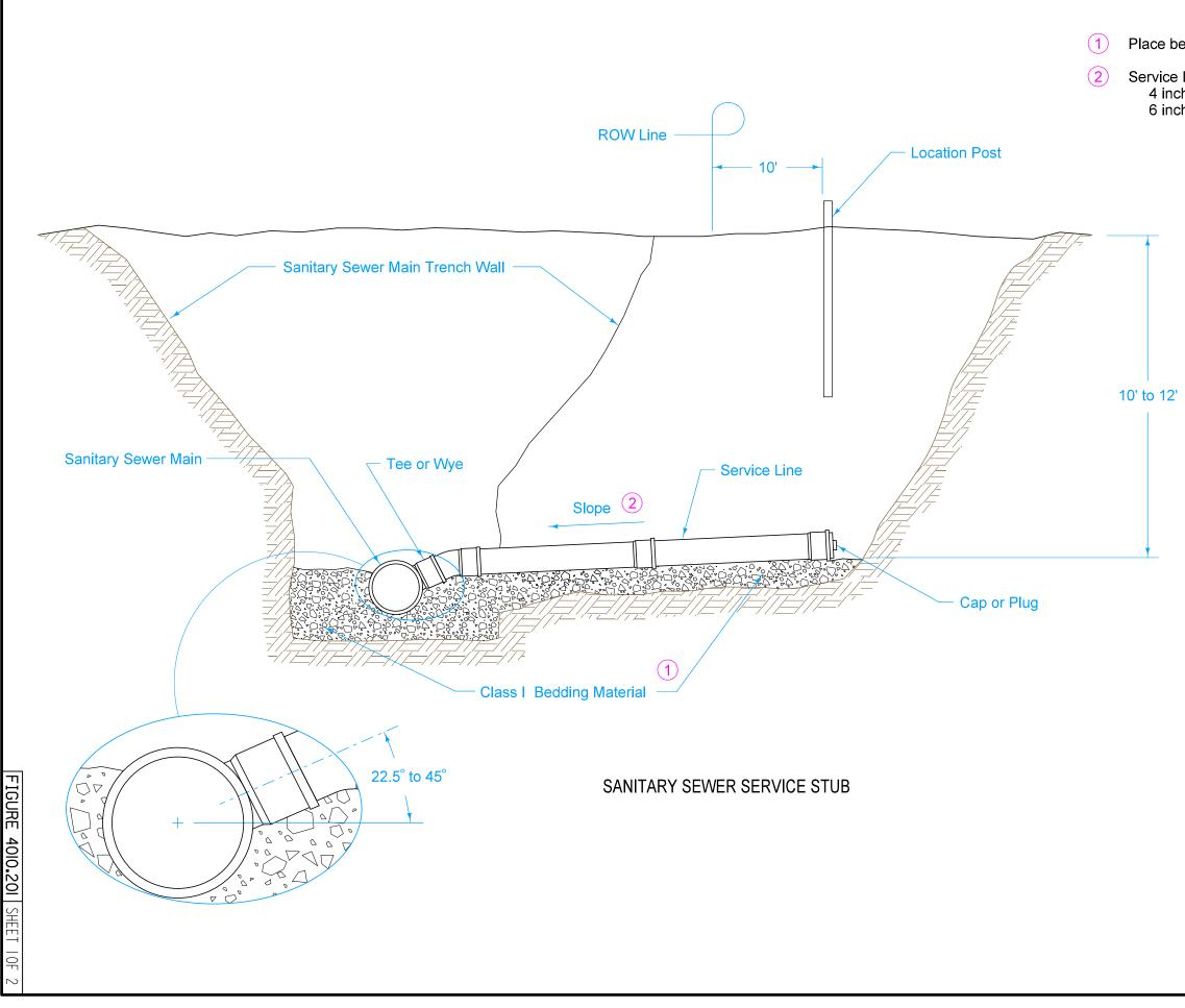
Place bedding and backfill material as required for sewer main.
