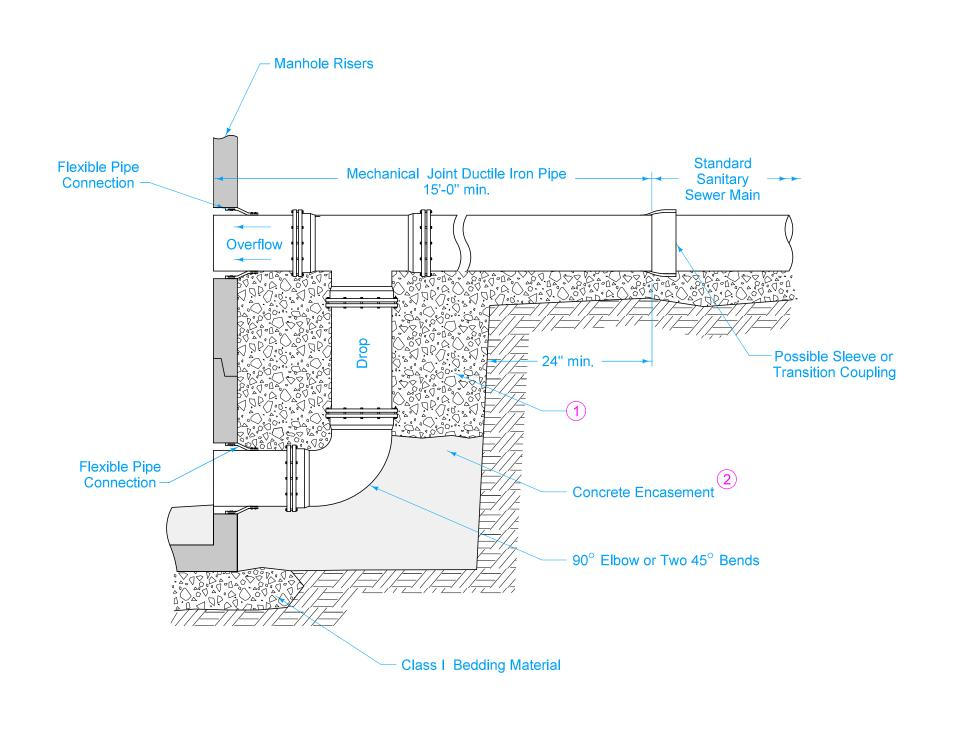
Construct drop and overflow from ductile iron pipe of same diameter specified for sewer main. Provide mechanical joints for all ductile iron pipe and fittings.
