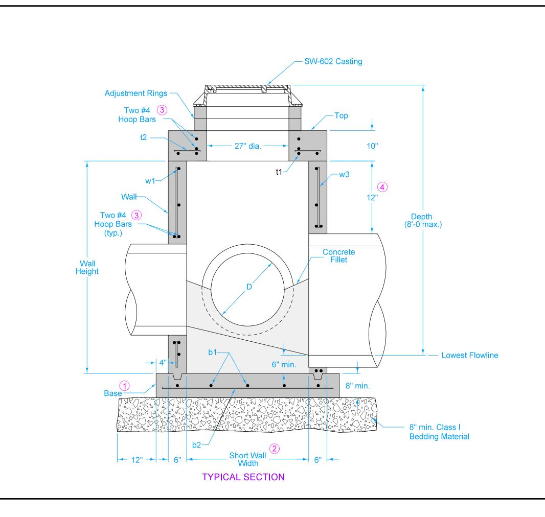
Adjacent walls may have different widths based upon pipe configuration, but structure must be rectangular.
