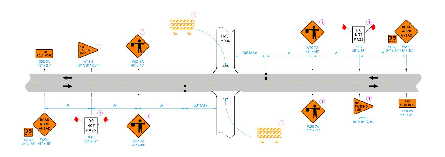
1 During nighttime hours or when the haul road is not in use, Type III Barricades shall be placed as shown and DO NOT PASS, NO PASSING ZONE and Flagger Symbol signs shall be covered or removed.
