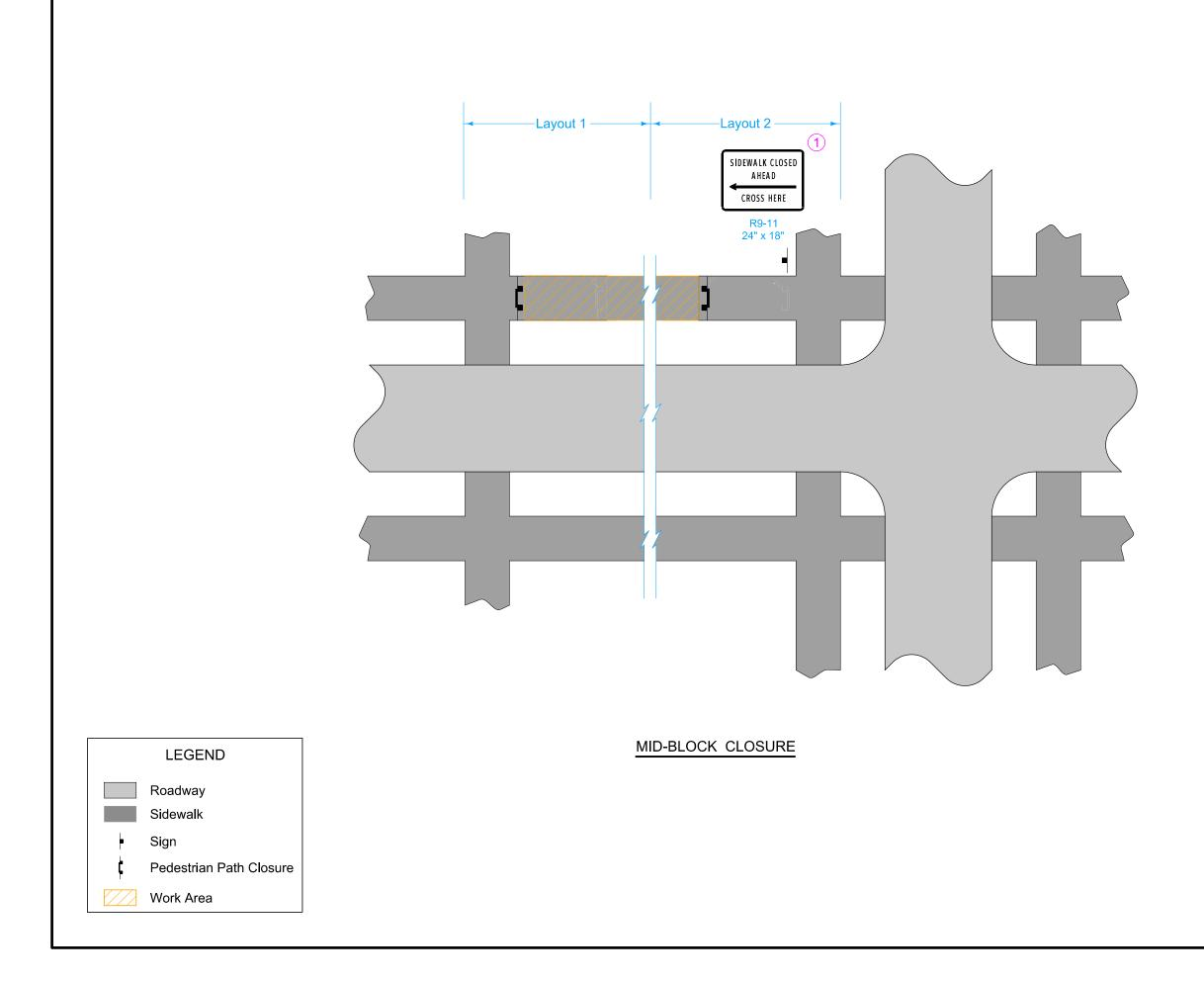
Omit "SIDEWALK CLOSED AHEAD CROSS HERE" (R9-11) sign when closure is at sidewalk intersection as shown in layout 1. (1
