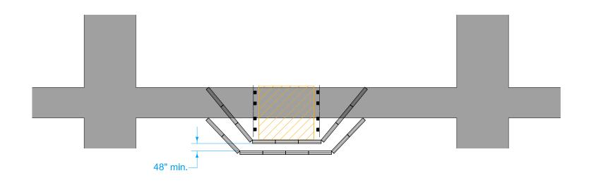
Acceptable materials and construction method for Pedestrian Channelizer will be defined in the contract documents. When Temporary Barrier Rail is specified as the Pedestrian Channelizer, Section 2528 of the Standard Specifications applies. For other types of Pedestrian Channelizers, the length of Pedestrian Channelizer installed will be measured in feet. Payment will be at the contract price per linear foot.
