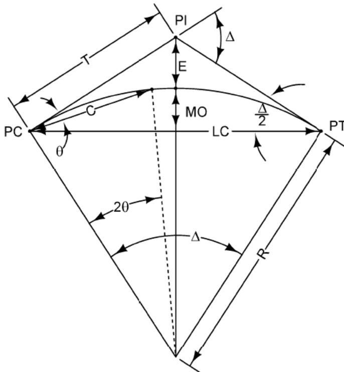
Figure 1: Components of a simple horizontal curve.
