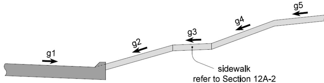
Type B and C entrances: g2, g4, and g5 should not exceed 14% and should be as flat as possible for Type B high volume traffic entrances.
