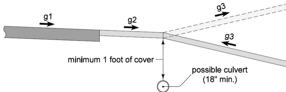
Type B and C entrances: g3 should not exceed 14% and should be as flat as possible for Type B high volume traffic entrances.
