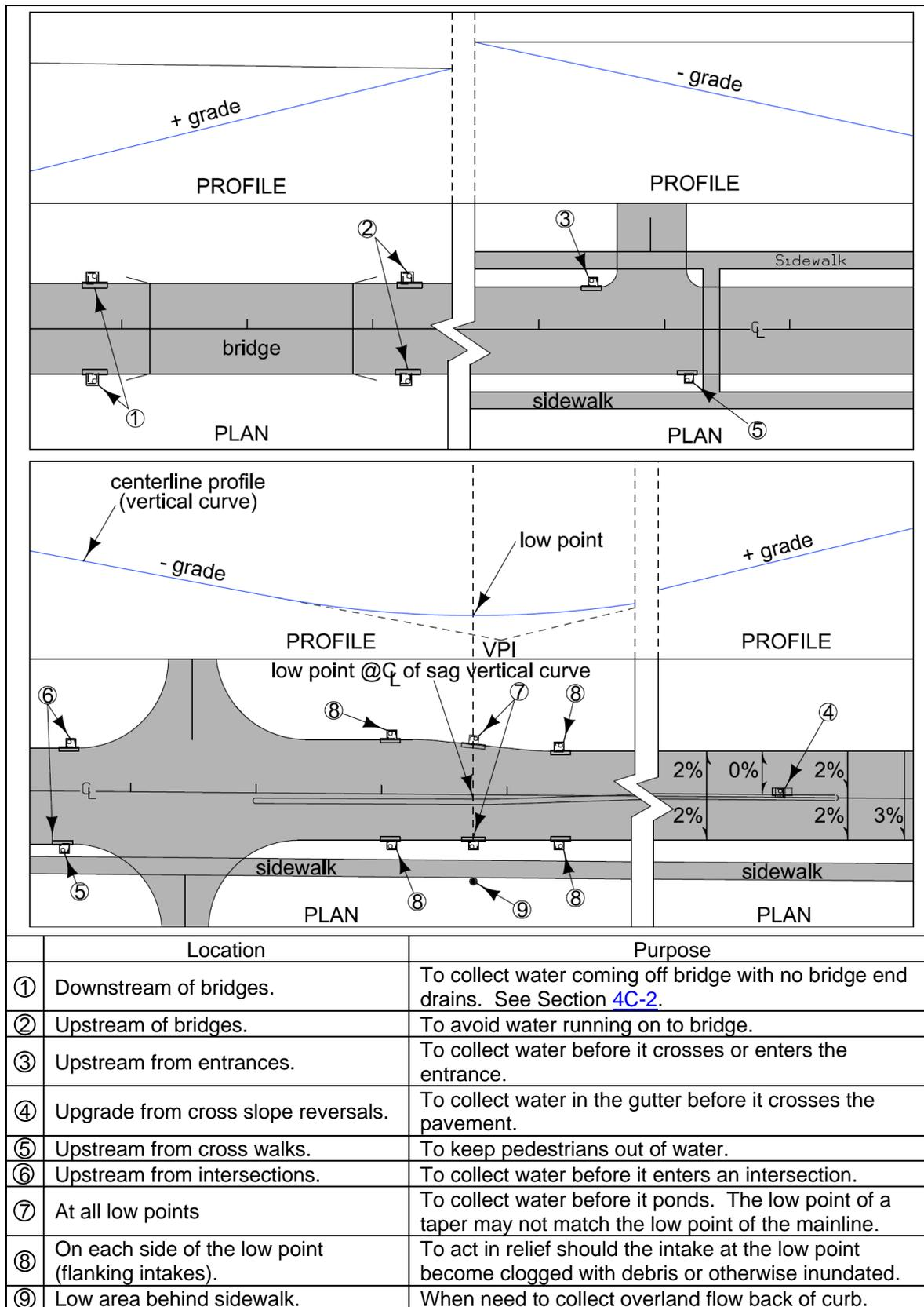
Figure 1: Plan and profile view of common intake locations.
