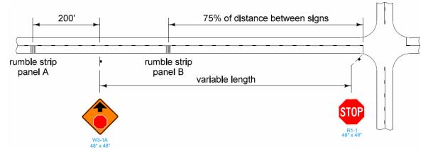
Figure 1: Rumble strip panel placement at stop signs.
