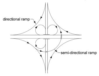
Figure 3: Semi-directional and directional ramps.
