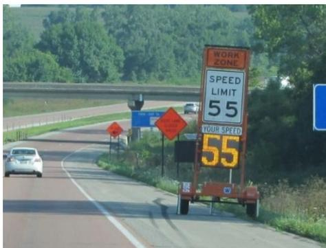
**Figure 1:** Speed feedback trailer sign.
