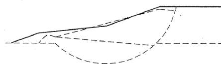
Rebuild with stability berm
