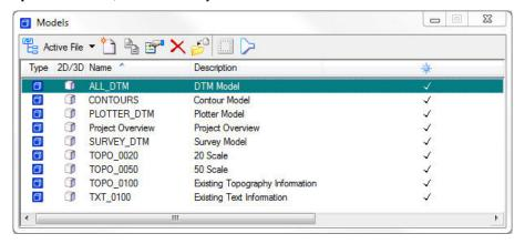
The *project#*.pho file contains only one photo text model, **TXT\_0100**, at 100 scale. Reference the **TXT\_0100** model to all necessary design models, where the appropriate information is to be copied, rotated and scaled to the design model.
