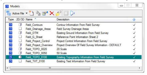
The *project#*.**sur** file contains only one survey text model, **Field\_TXT\_0100**, at 100 scale. Reference the **Field\_TXT\_0100** model to all necessary design models, where the appropriate information is to be copied, rotated and scaled to the design model.
