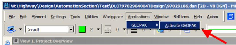
After GEOPAK has been activated, access the GEOPAK **Survey** menu from the MicroStation menu by selecting **Applications > GEOPAK > SURVEY > Survey**, as shown at the right.
