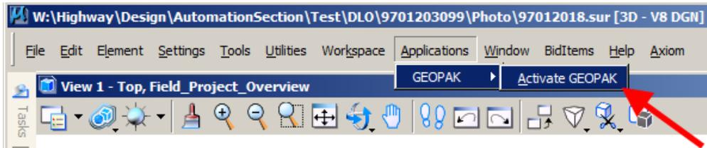
2.) You must tell GEOPAK where the ".gpk" file containing the station and offset information is located. This is done by changing the user preferences. From the main MicroStation tool bar, *select*
