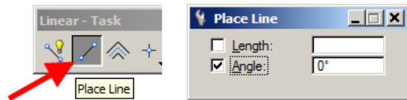
If using the place line tool, the angle option should be checked (☑), and the active angle should be set to 0 (zero), as shown above.
