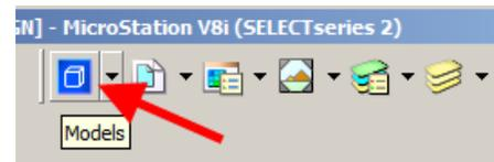
In the **Models** dialog, switch to the **Field\_TOPO\_0100** model by *double-clicking* the model name in the list, as shown at the right.
