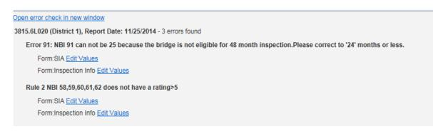
A management report called Extended Inspection Frequency Report can be run and used to determine if a bridge is eligible or not eligible for an extended inspection interval. If the bridge passes all the rules except rule 17 (An In-depth inspection was not done at the current inspection and the last value of NBI 91 was not 48) the bridge may be eligible for an extended inspection interval of up to 48 months at the next inspection if an in-depth inspection is performed.
