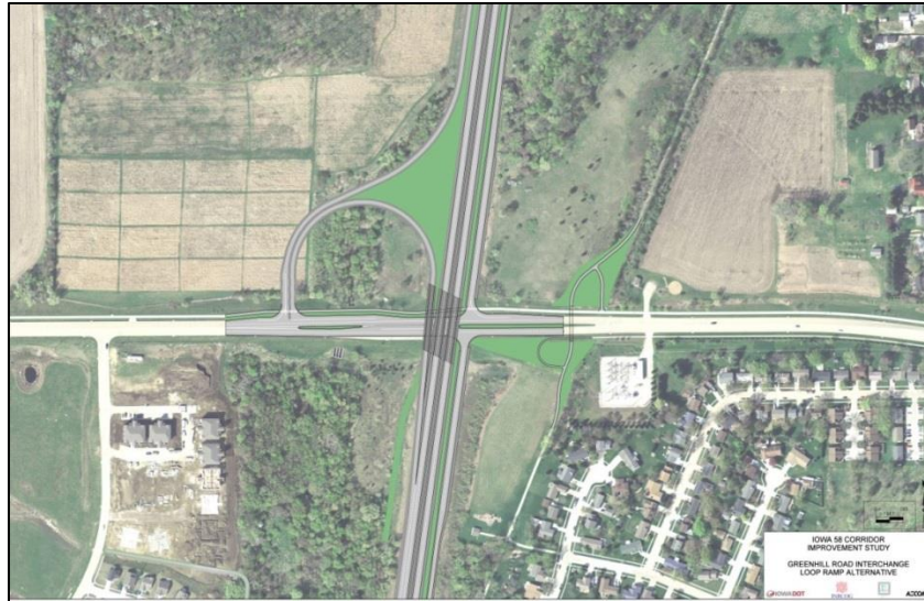
Loop Ramp Alternative at Greenhill Road
