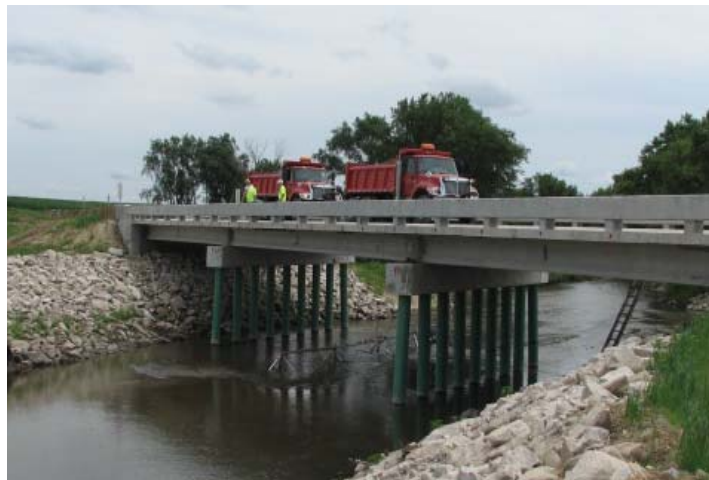
Figure 2.11 Static test (Load Case 1)
