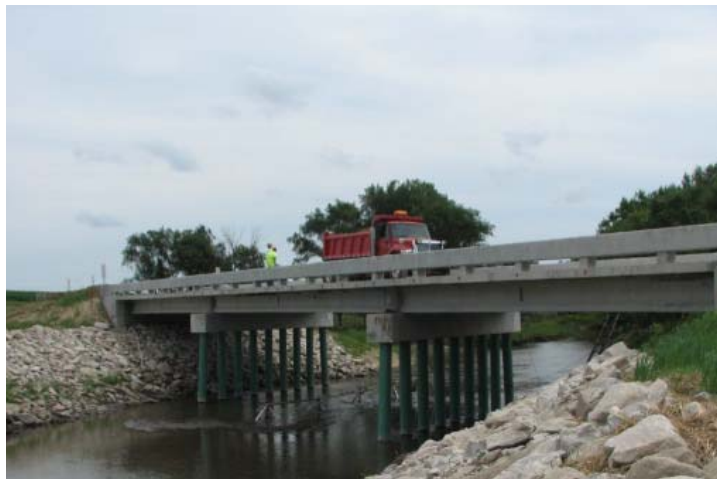
Figure 2.13 Static test (Load Case 3)
