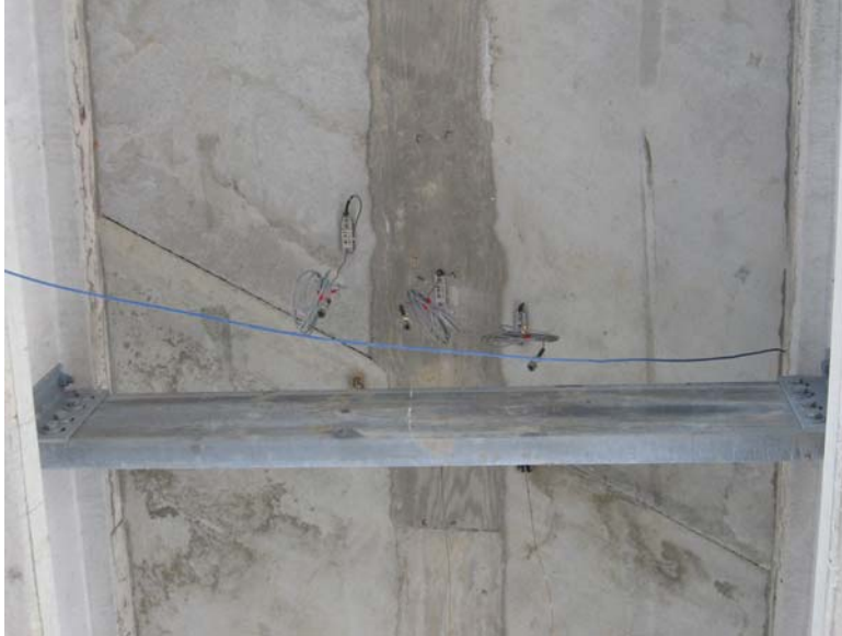
Figure 2.4 Instrumentation layout at closure joint
