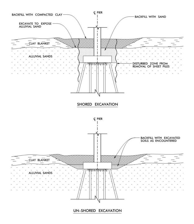
Figure 1: Pier Nos. 1 and 2 Excavation and Backfill Detail
