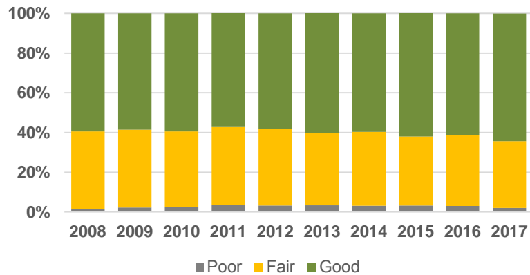
Non-NHS Pavement Condition State PCI Metric
