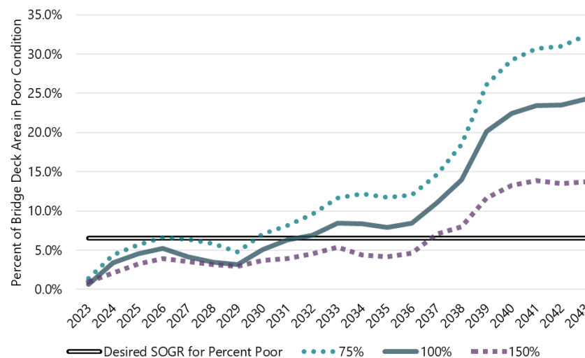
Figure 4.4: NHS bridge condition performance scenarios for federally defined poor condition
