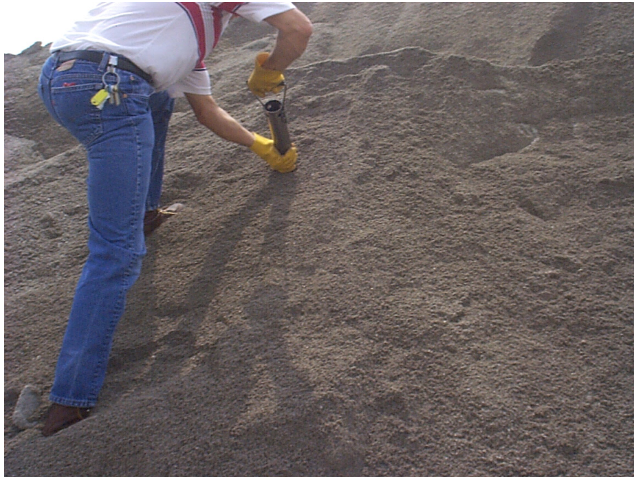
Stockpile sampling using a sand probe.
