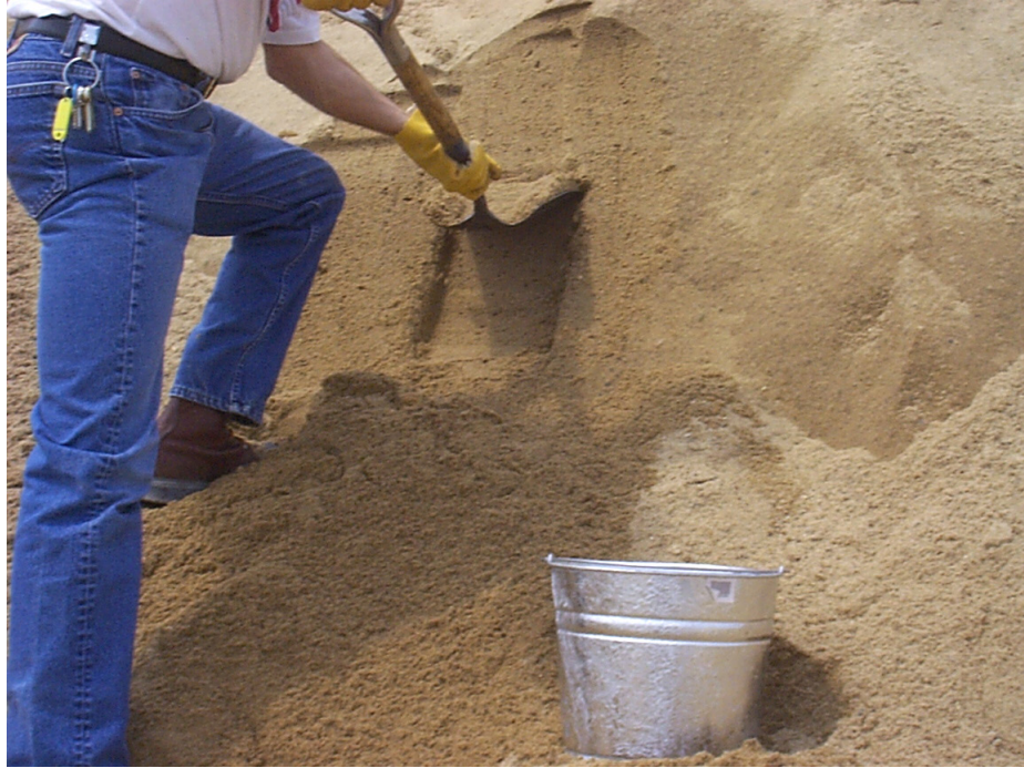
Stockpile sampling using a shovel.
