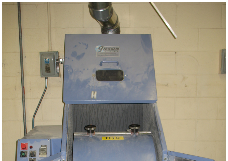
Los Angeles Abrasion test machine
