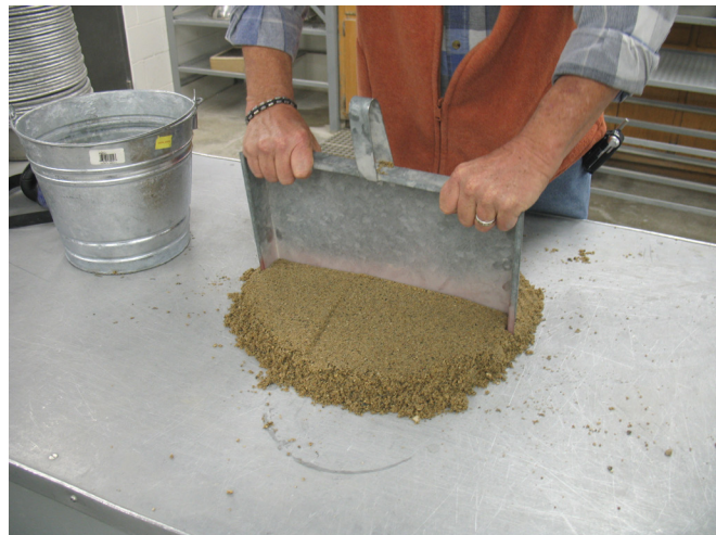
Quartering using straight edge.
